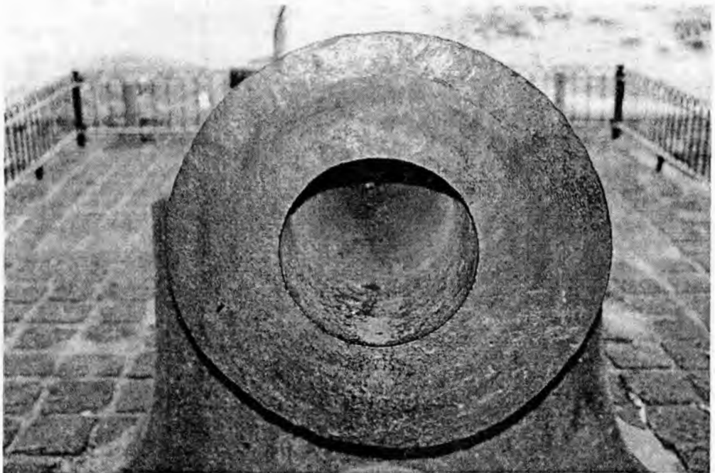
Fig. 5: Front end of the cannon showing that three iron rings have been forged on top of each other successively in order to produce the thickness of the cannon cross section.
